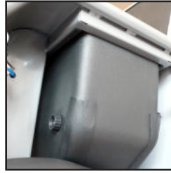
Insulated pellet hopper with 9kg (19.84 lb) capacity
